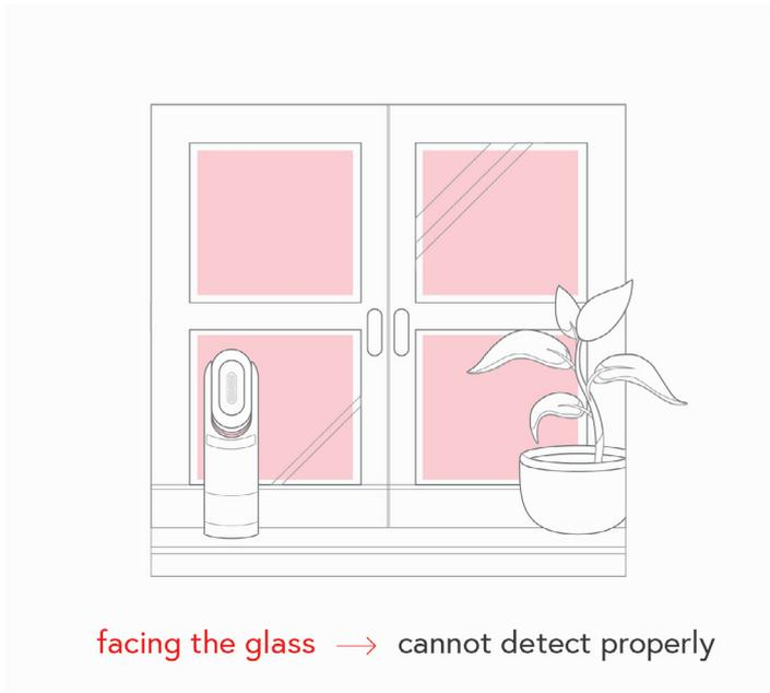
**a.** The camera cannot properly detect events through the glass. Don't place it behind or facing a window/glass
